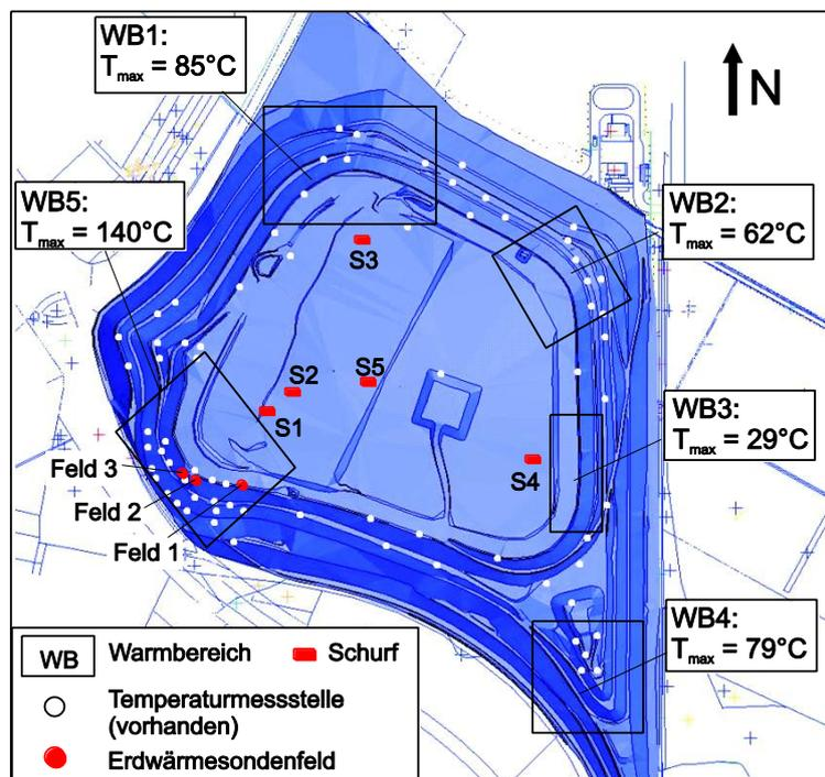
Figure 1: Dump Site (Position of Hot Spots (WB), Borehole Heat Exchangers and Test Pits)
