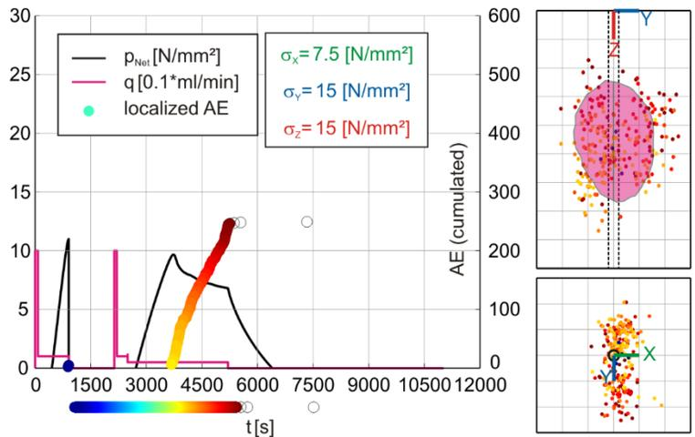
**left: Injectionrate, -pressure and cumulated AE right: Fracture area and AE projected into plane Y-Z and X-Y**
